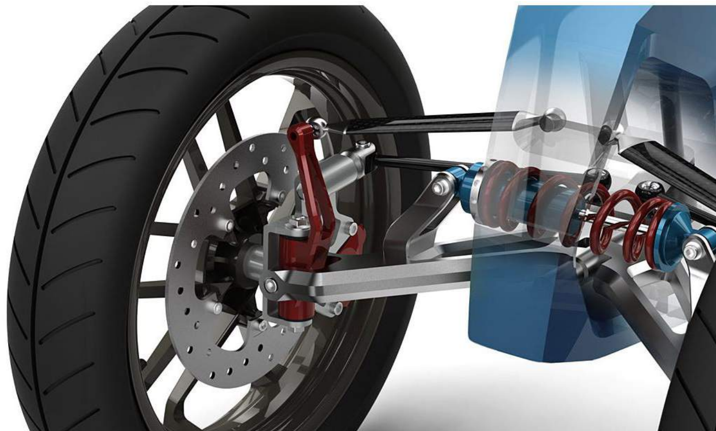
(54) Title: A THREE-WHEELED CAR FRAME CAPABLE OF INCLINING WHEN HANDLING A CURVE
