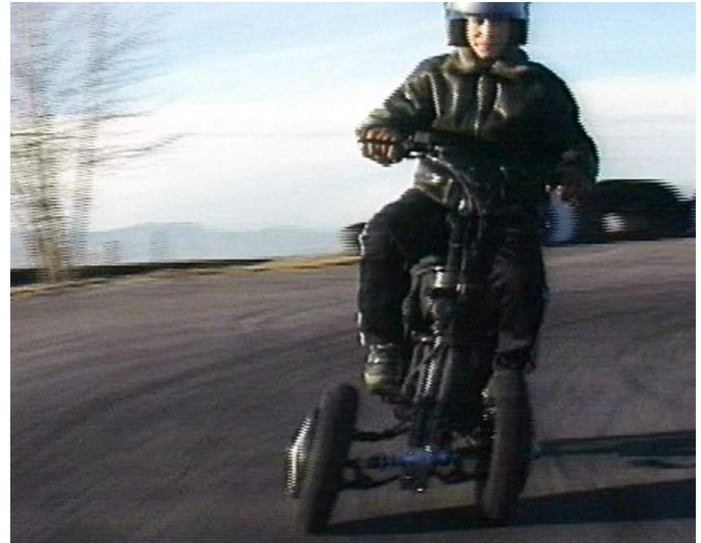
(54) Title: A THREE-WHEELED CAR FRAME CAPABLE OF INCLINING WHEN HANDLING A CURVE
